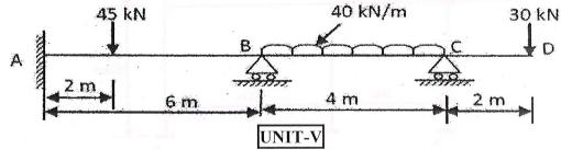
9. Find the required value of plastic moment capacity at collapse load for the continuous 12M beam shown below? Take AB=2Mp; BC=1.5Mp; CD=Mp.
